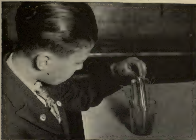
FIG. 161. Water can be separated into two gases by a current of electricity.
